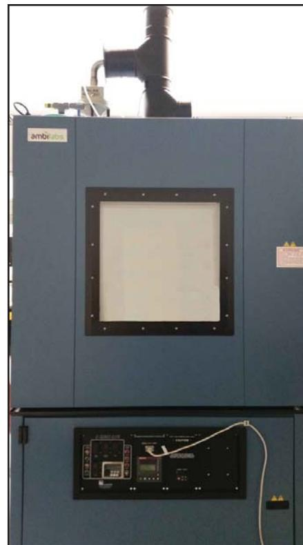
*Above: Chamber front with particle generator mounted at the top.*
