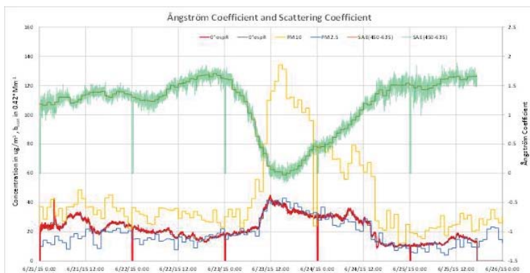
(Above) On 6/23/15, the Ångström Exponent (green) decreases, revealing the coarse particle influence from a Sahara Dust event in Atlanta, GA. Collocated PM measurements show a corresponding increase in PM10 concentration (yellow). The red scattering coefficient (635 nm) follows mostly the PM2.5 concentration and can be scaled with a user defined factor to get a PM2.5 estimate. The 1 minute Nephelometer data show the exceptional time resolution of the instrument.
